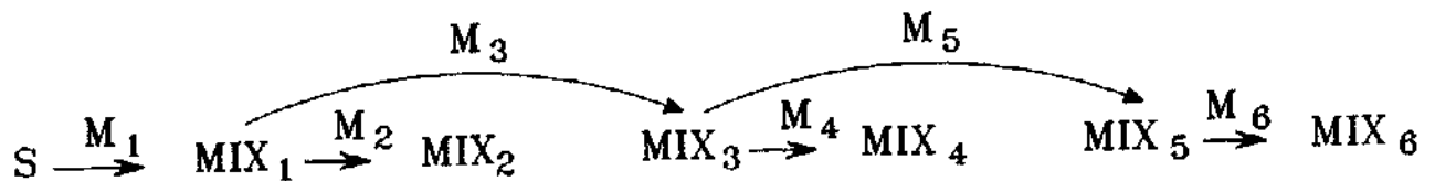
Fig. 12: Skip 1 MIX scheme operated in the mode "skip as few as possible"
